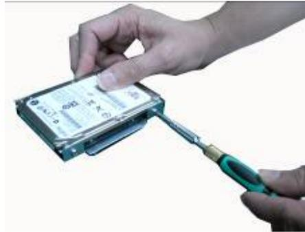
**Step 6** Install and fix the HDD through the bottom & side, next, plug the power cable in HDD.
